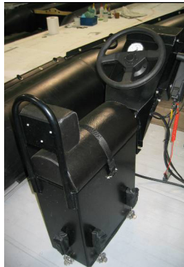
Jockey seat with a mounted steering pod
